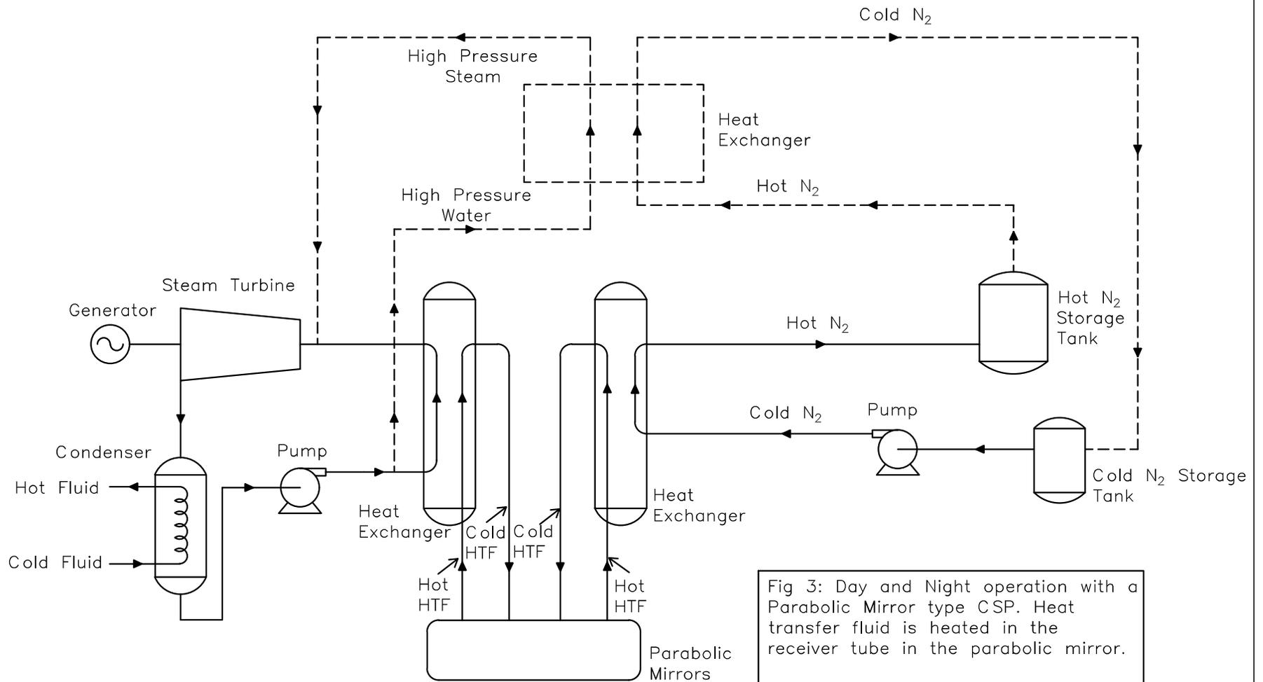
Fig 3: Day and Night operation with a Parabolic Mirror type CSP. Heat transfer fluid is heated in the receiver tube in the parabolic mirror.
