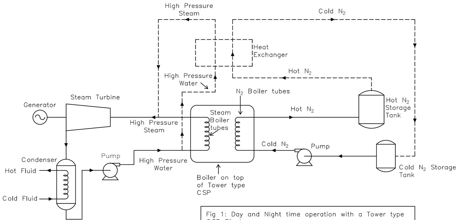
Fig 1: Day and Night time operation with a Tower type CSP Plant.
