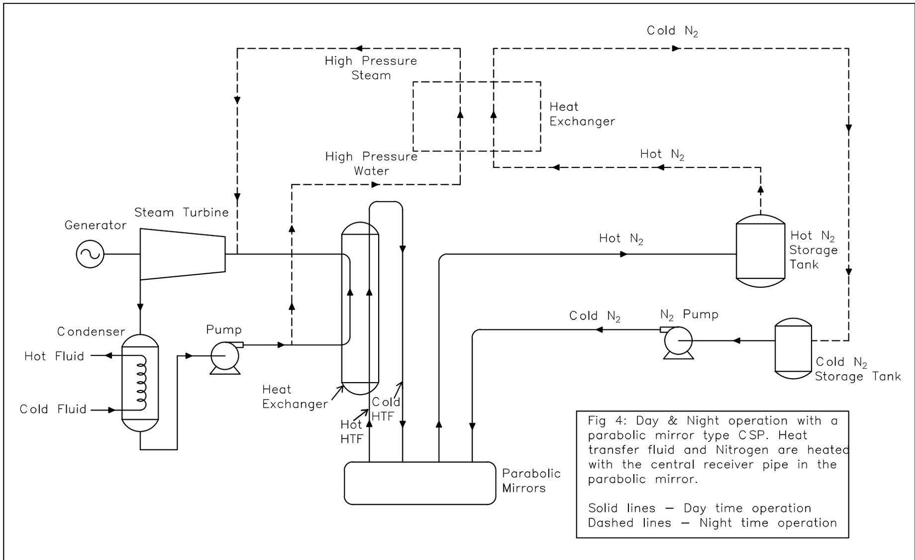
Fig 4: Day & Night operation with a parabolic mirror type CSP. Heat transfer fluid and Nitrogen are heated with the central receiver pipe in the parabolic mirror.
