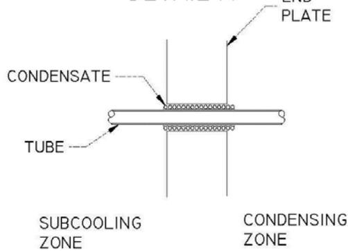
ONE AND ONLY BARRIER BETWEEN CONDENSING AND SUBCOOLING ZONE
