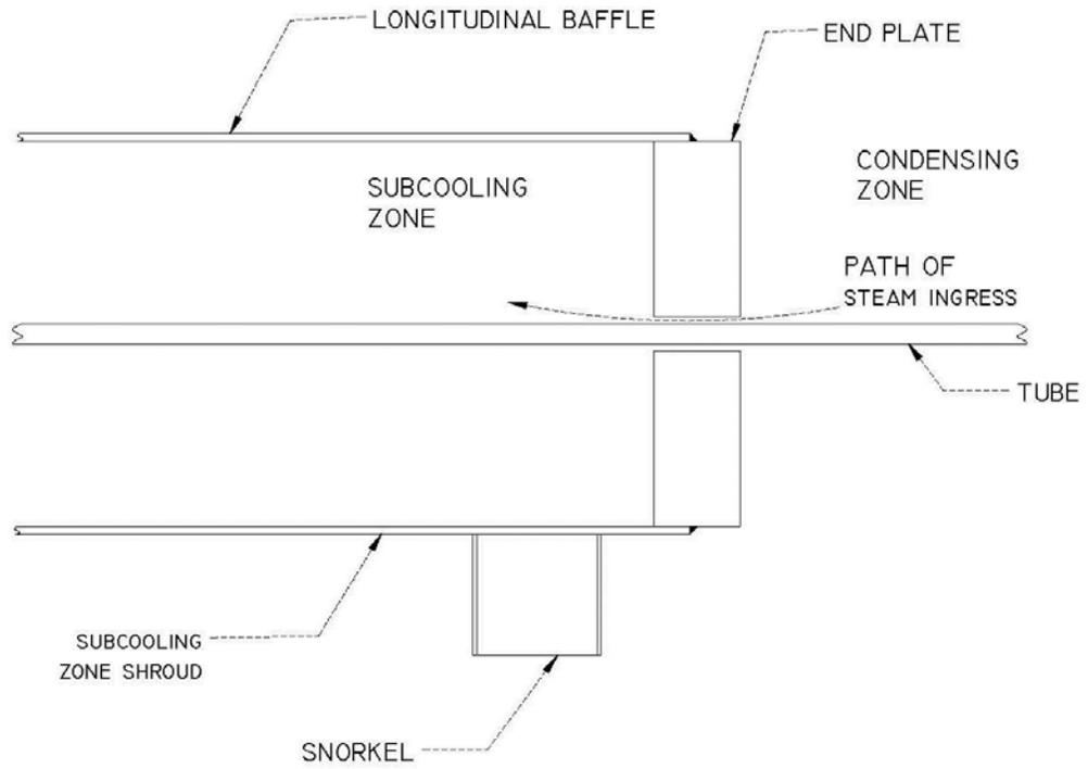
FIGURE 4: SINGLE END PLATE DETAIL
