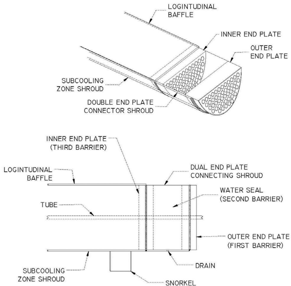
DUAL END PLATE WITH WATER SEAL OFFERS TRIPLE BARRIER TO LEAKAGE OF STEAM INTO SUBCOOLING ZONE
