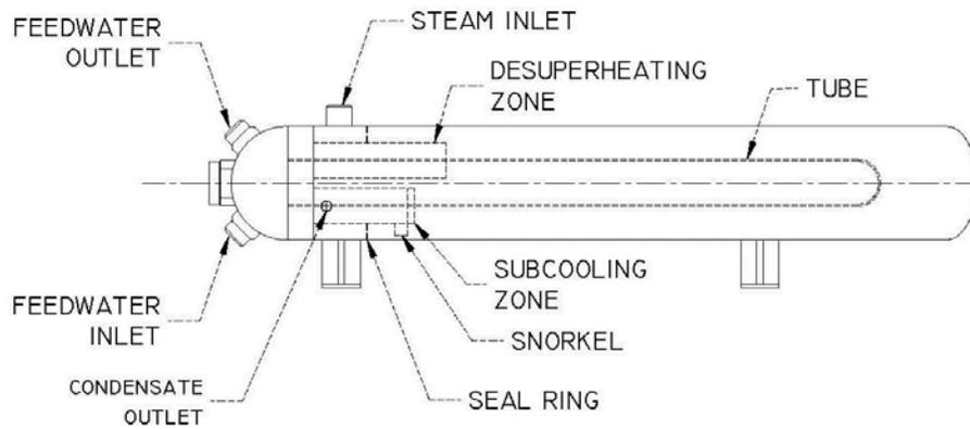
FIGURE 1: HIGH PRESSURE FEED WATER HEATER
