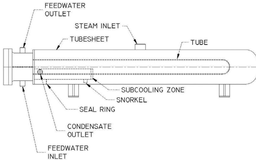
FIGURE 2: LOW PRESSURE FEEDWATER HEATER
